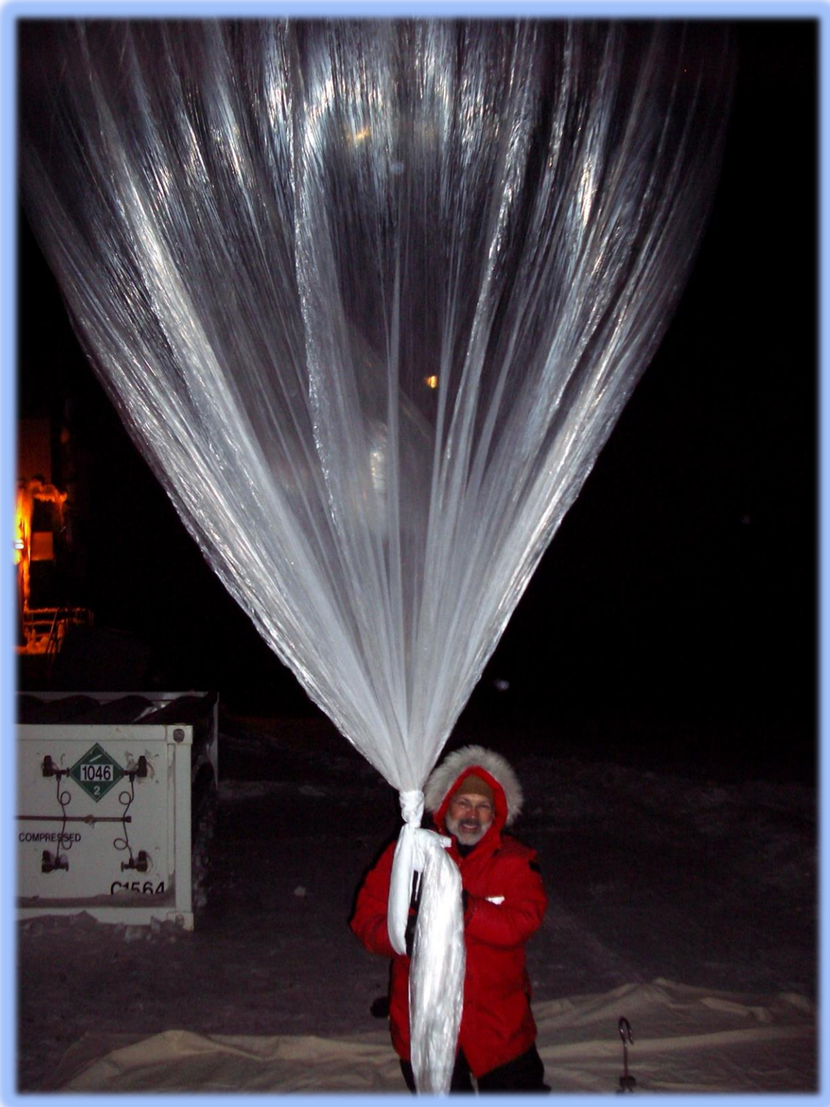
Figure 1. About to launch an ozonesonde at McMurdo, Antarctica, August 25, 2004.
