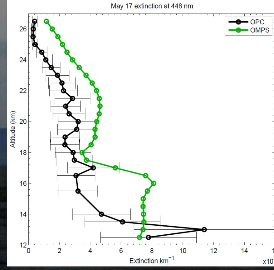
Comparison between the OPC and OMPS estimates of extinction for both March 26 and May 17 of 2013 at two additional wavelengths- 448 nm (left) and 869 nm (right). The data aspect ratio is held constant in all extinction plots, so that relative magnitude between different wavelengths can be evaluated.
