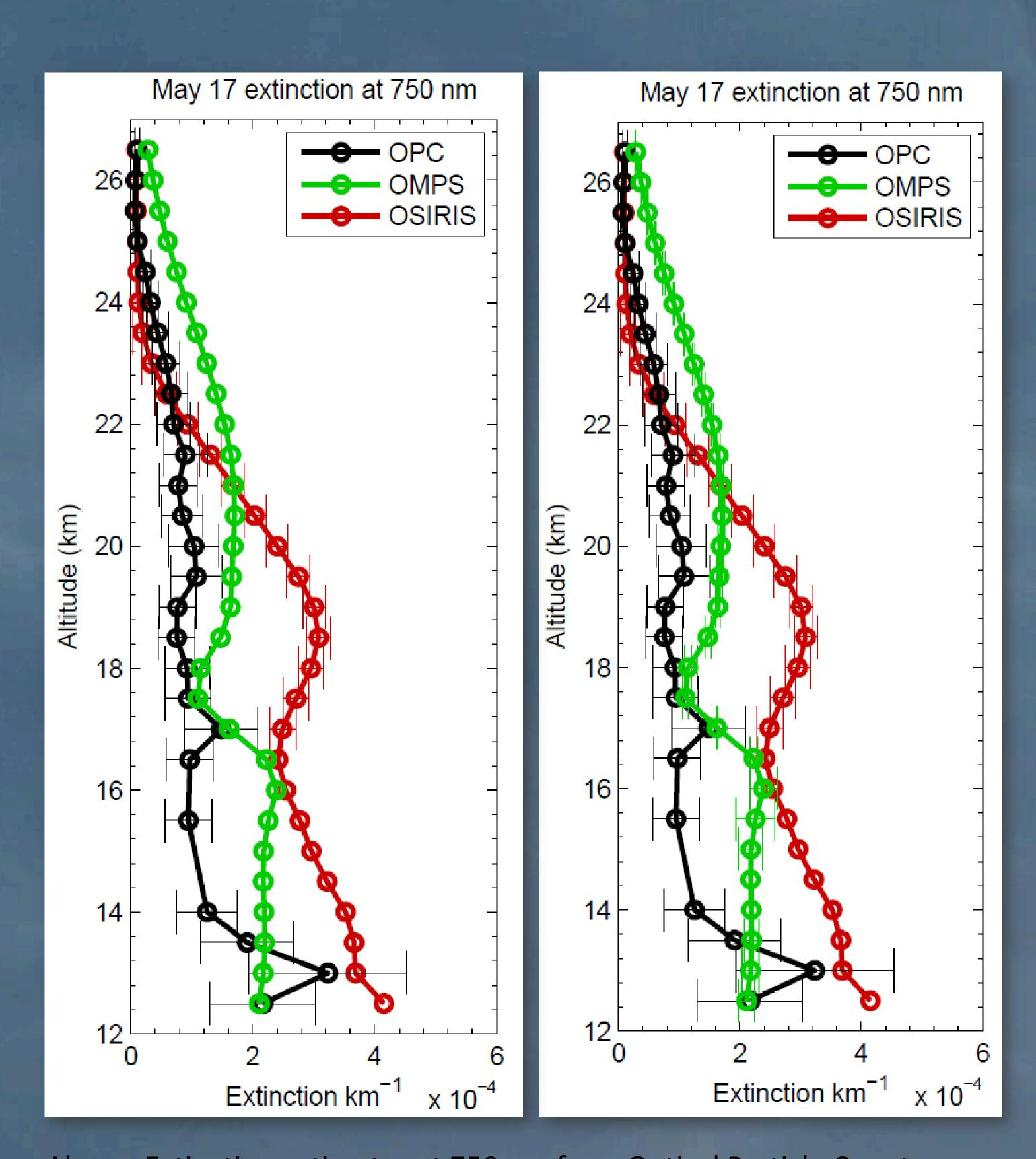
Above: Extinction estimates at 750 nm from Optical Particle Counter compared with remote sensing instruments OMPS and OSIRIS for March 26 and May 17 of this year. The in-situ measurements were made over Laramie, WY (42° N), and both satellite profiles are from approximately the same location. In the case of the OPC data, the extinction at each altitude is calculated from the size distributions shown to the right, with the relationship:
