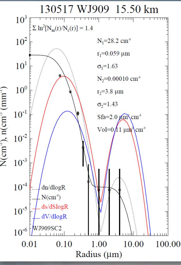
Bimodal lognormal size distributions fit to the OPC concentration measurements at two example altitudes, 14.5 km (top) and 19.5 km (bottom).  $N_i$  is total number concentration,  $r_i$  the median radius, and  $\sigma_i$  the distribution width.
