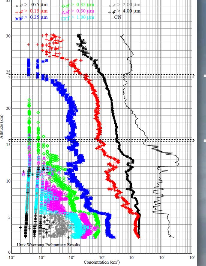
Cumulative concentration measurements from the Optical Particle Counter for aerosol with radius ≥ 0.075, 0.15, 0.25, 0.35, 0.5, 1.00, 2.00, and 4.00 μm.
